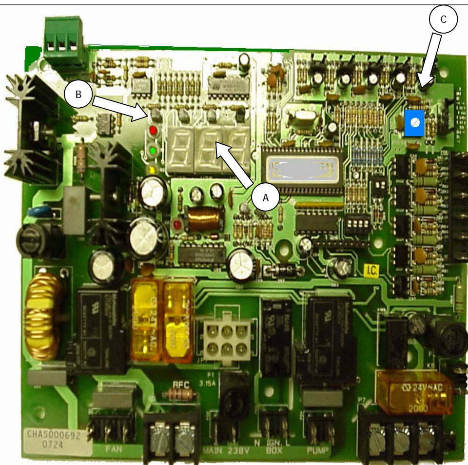
Figure 2 - The S-50 Electronic Control Board
